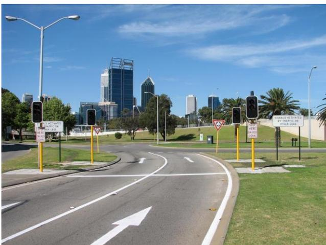
Point Lewis Rotary meter signal in "off-state"
