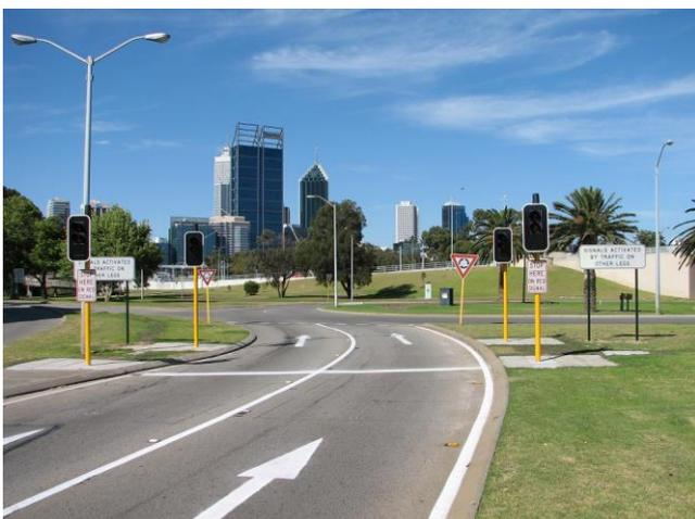
Installed Point Lewis Rotary meter signal in "off-state"
