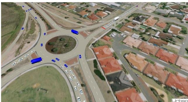
Simulation of roundabout metering in Canning Vale
